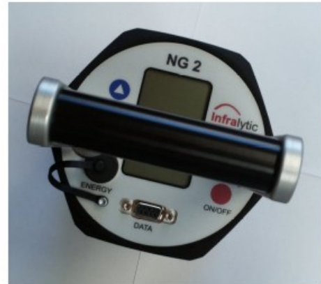
Figure 2: Handle of sensor perpendicular to the rolling direction
