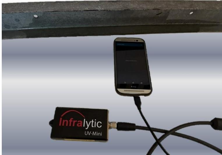
The Infralytic UV-Mini is an additional measuring device for the Infralytic hand-held device NG3. We designed the UV-Mini especially for measuring the oil layer thickness on metallic surfaces - for complex, deformed or pressed 3D components.
