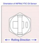
*Some steel surfaces but especially aluminum surfaces are structured very in-homogeneously, due to the rolling process. Therefore, make sure that the sensors handle is positioned perpendicular with regard to the rolling direction, when taking a measurement on these surfaces.*
